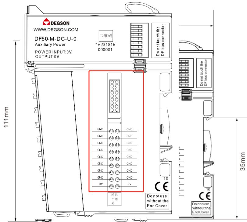
Each of the 16 channels can provide a rated voltage of 0VDC for external loads.
